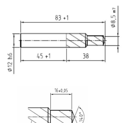
Solid carbide step drill, coated Shank DIN 6535 HA 8,5 x 16/90° x 12 x 83 mm, Z=2 8,5x90°x12x83
