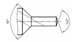
Solid carbide step drill, coated Shank DIN 6535 HA 2x5,5/90°x20x6x80mm; Z2
