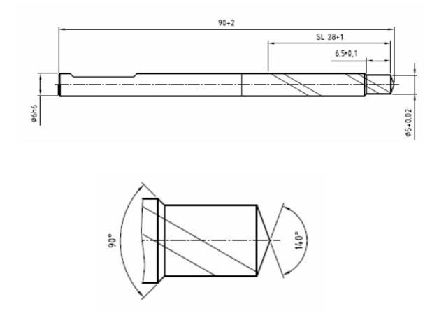
Solid carbide step drill, coated Shank DIN 6535 HB long 5x6,5/90°x28x6x90mm;Z2
