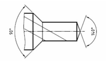
Solid carbide step drill, coated Shank DIN 6535 HB long 3x5,5/90°x25x6x80mm; Z2
