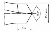
Solid carbide special center drill Shank DIN 6535 HA 5 x 18 x 60 mm, Shank14 mm, coated 5x18x60
